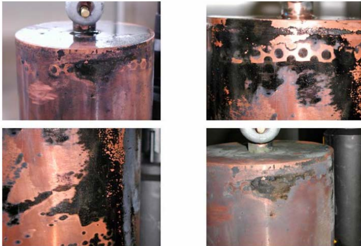
Figure 6-12. Appearance of the surface of the copper canister. The chain-like pattern on the surface at the top of the canister corresponds to the contact area with the strip of plastic insulator that was placed between the copper canister and the inner surface of the support cage.
